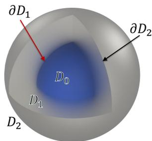
Fig. 1. Geometry of the model: plane wave scattering on the sphere with transparent core (refractive index 1.4,  $r_1 = 3nm$ ) and silver shell ( $r_2 = 6nm$ ) is considered.
